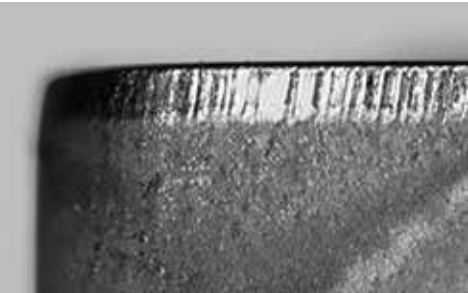
Abrasion on flank, normal wear after a certain machining time.
